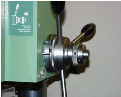
Picture 2. Inserted coupling
